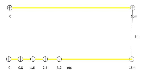
4-To align the second cones line parallel to the first one, find the meeting point between the 3m measure taken from the last point of the first cones line (the center of finish line) and 16m. Mark the intersection
