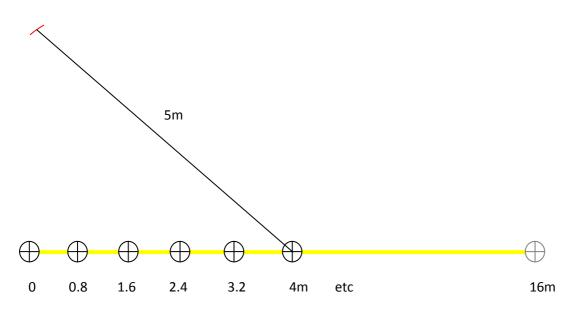
3- From the zero point measure 3m, find intersection with the previous arch and mark it. This is the zero point of the second line. This point is at 3m distance from the zero of the first cone line and the line that meets the two zero points is perpendicular to the first cone line.
